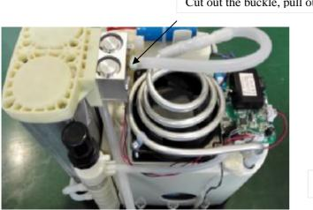
Cut out the buckle, pull out the pipeline
